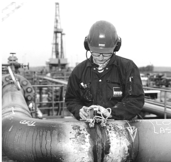
Figure 14: ToFD inspection in the field
