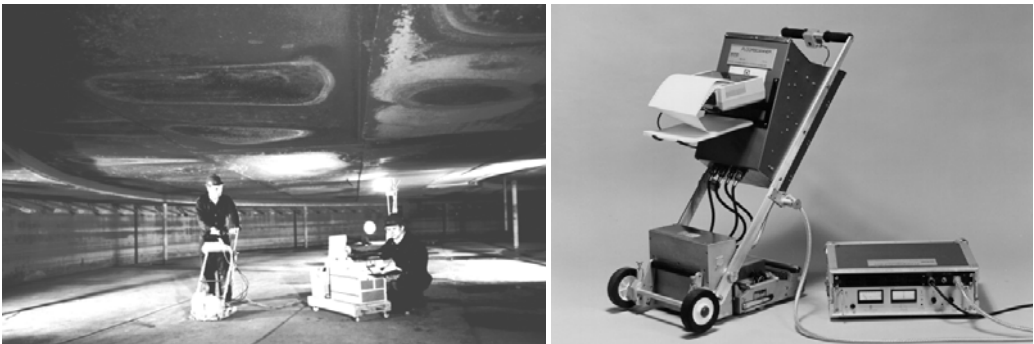
Figure 10: Left: Prototype Floorscanner of APS inside a storage tank. Right: The Mk1a Floorscanner as it was built for commercial use
