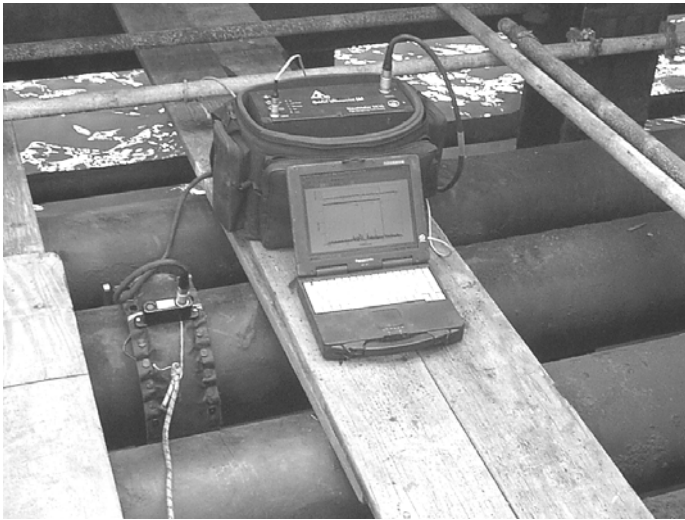
Figure 15: Guided Waves equipment in the field
