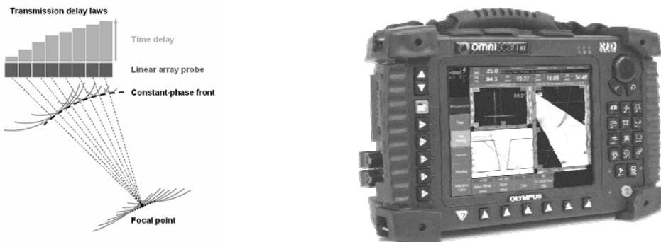
Figure 18: Left, the principle of Phased Arrays. Right, an R/D tech Omniscan portable phased array system
