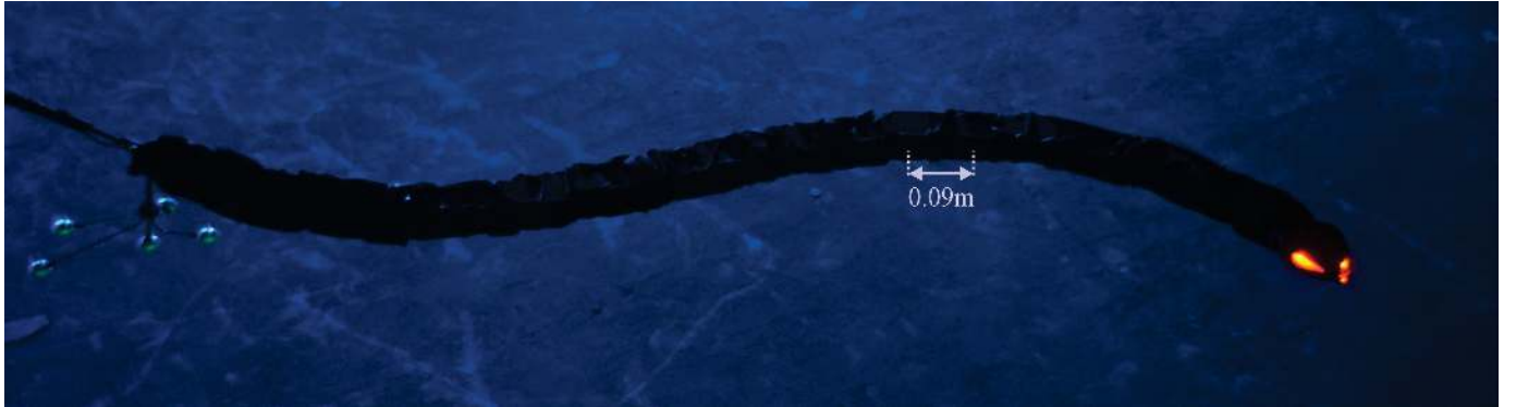
Fig. 6. The underwater snake robot Mamba in the pool with the markers attached on the tail for position measurements.
