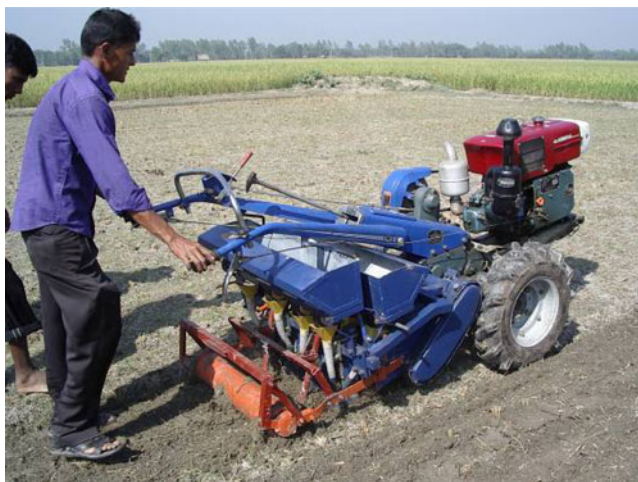
Fig. 2 Versatile multi-crop planter (VMP), with seed and fertilizer delivery attachments fitted to a Chinese-made two-wheel tractor (power tiller), sowing lentil by strip tillage after rice, Bangladesh, November 2009. The machine can be easily modified to sow by zero tillage (all rotary blades removed), full tillage (all rotary blades present), and to sow on beds
