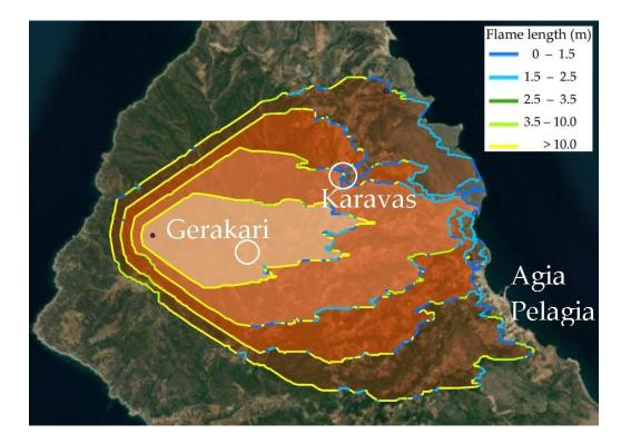
**Figure 6.** A fire spread simulation example, using the G-FMIS fire simulation system, in the north part of Kythira (Karavas and Gerakari settlement) under a west wind, showing fire perimeter growth (in four hourly steps) and flame length (m) along the perimeter color-coded in five classes.
