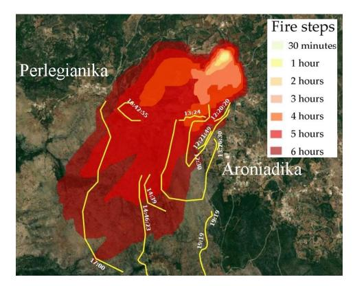
**Figure 5.** Comparison of the actual evolution of the perimeter of the fire of 4 August 2017 in Kythira (Pitsinades fire), which started at 10:55 am, with the simulated growth of the perimeter at regular intervals with the G-FMIS system, using the actual meteorological conditions of that day and the fuel map of Figure 3.
