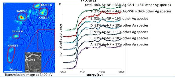
To have a better understanding of Ag internalization mechanisms, a root cross-section was analyzed by full-field XANES (Figure 3C, D, Table 1). This technique permits to obtain 2D speciation of an element
