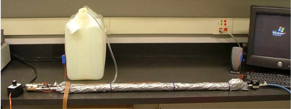
Figure 7.2: Overview of Setup for Tube-Side Heat Transfer Experiments
