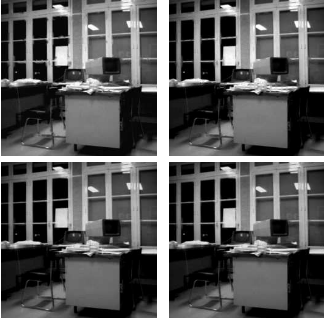
Figure 4: Interpolation of the image in Fig. 3. Top left: Cubic interpolation by the MATLAB procedure 'griddata' (PSNR=30.18, err_2 = 7.89 , err_1 = 1.51 ). Top right: algorithm A, (PSNR=31.61, err_2 = 6.69 , err_1 = 1.36 ). Bottom left: algorithm B, (PSNR=34.08, err_2 = 5.03 , err_1 = 0.93 ). Bottom right: algorithm C, (PSNR=33.98, err_2 = 5.09 , err_1 = 0.97 ). The images at the top contain artefacts, in particular at the left window side. The algorithms at the bottom show a better performance and do not introduce these artefacts.
