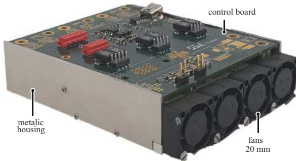
Fig. 7. Inverter hardware prototype with dimensions 99.6 \text{ mm} \times 80 \text{ mm} \times 23.7 \text{ mm} . A power density of 5.8 \text{ kW/dm}^3 ( 95 \text{ W/in}^3 ) is achieved.
