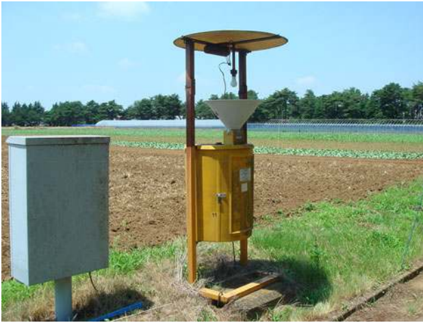
Fig. 3 A light trap that uses an incandescent light. Data on numbers of single insect species are used to forecast pest outbreaks
