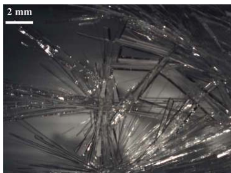
Fig. 1 Crystal shape of menthol after a slow sublimation condensation process under a secondary vacuum.
