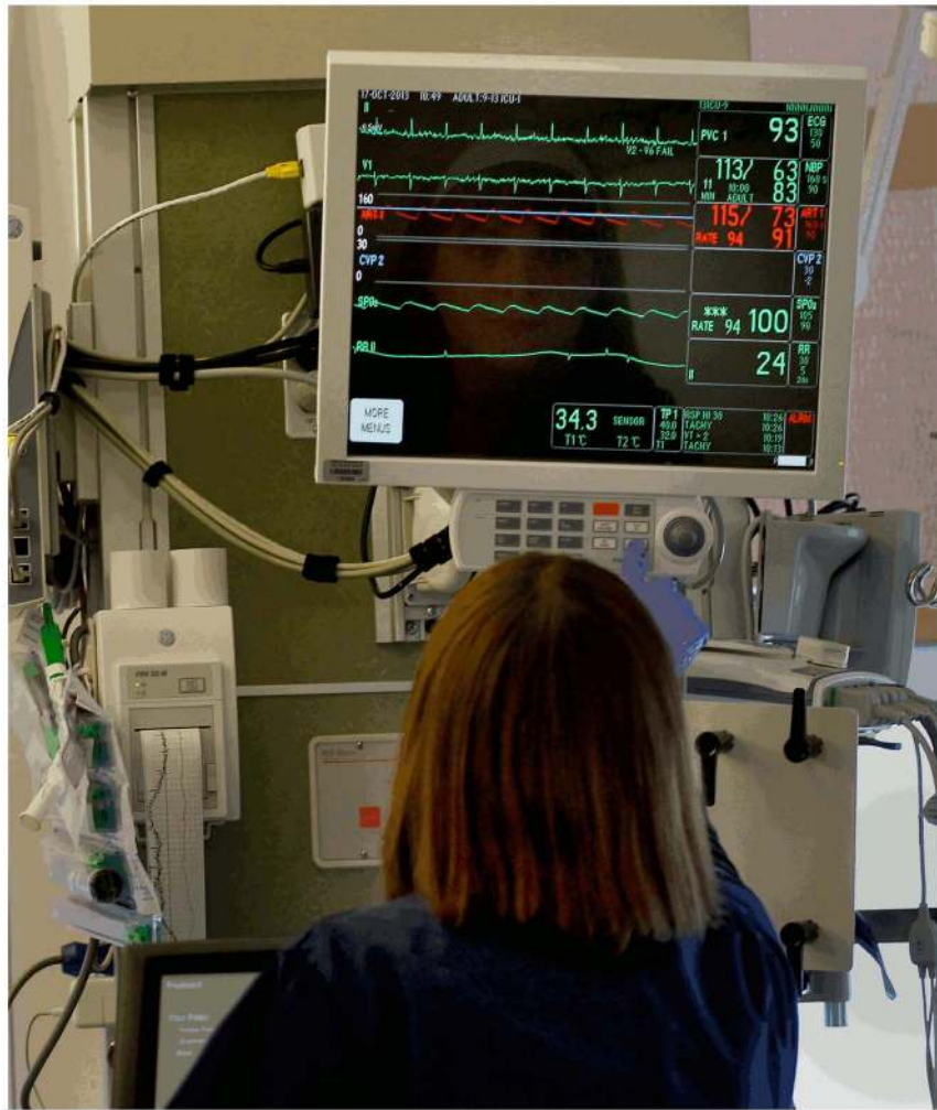
Figure 1. Physiologic monitor device in Intensive Care Unit. Bedside patient monitor (GE Healthcare, Milwaukee, WI) displays multiple physiologic waveforms and vital sign measurements. The nurse pictured here gave written informed consent to publish this photograph supplied by the San Francisco Chronicle newspaper (with permission) for their story on alarm fatigue at: http://www.sfgate.com/health/article/Hospitals-look-to-reduce-danger-of-alarm-fatigue-4918018.php . doi:10.1371/journal.pone.0110274.g001
