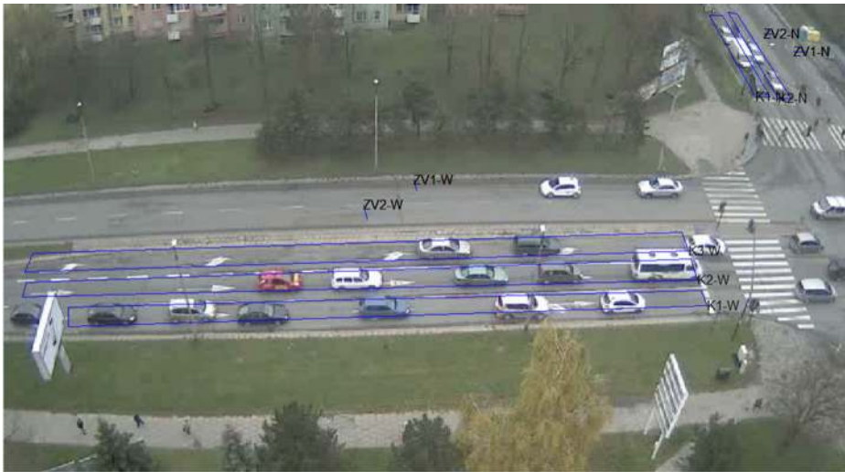
Fig. 2 Scene configuration of the Northern camera. There are 5 queue areas (denoted K) and 4 virtual lines (ZV) defined
