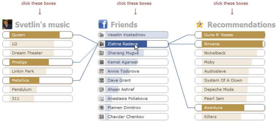
Figure 1. The TasteWeights system as used in the online user experiment. This is the inspection phase of the “full graph” condition. Users can click on items, friends and recommendations to see the links between them. The inspection phase of the “list only” condition shows the rightmost list (recommendations) only.
