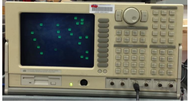
Figure 2. Stanford Research Systems SR780 2-Channel Network Signal Analyzer
