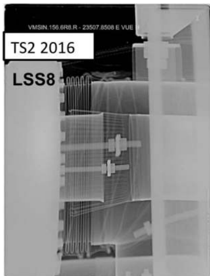
Figure 8: LSS8 vacuum module shows that a missing spring has caused rf fingers to no longer be in contact. This can cause heating due to the excitation of resonant modes with frequencies close to the beam spectrum.
