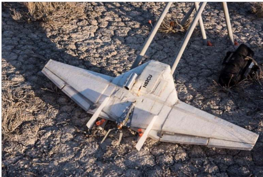
Figure 2. DH2 sUAS ready for launch at DPG during the IDEAL campaign.
