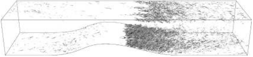
FIGURE 6. Iso-value of the Q -criterion ( Q = \frac{1}{2} [|\boldsymbol{\Omega}|^2 - |\mathbf{S}|^2] with \mathbf{S} = \frac{1}{2} [\nabla \mathbf{u} + (\nabla \mathbf{u})^T] and \boldsymbol{\Omega} = \frac{1}{2} [\nabla \mathbf{u} - (\nabla \mathbf{u})^T] ) for the whole simulation domain.
