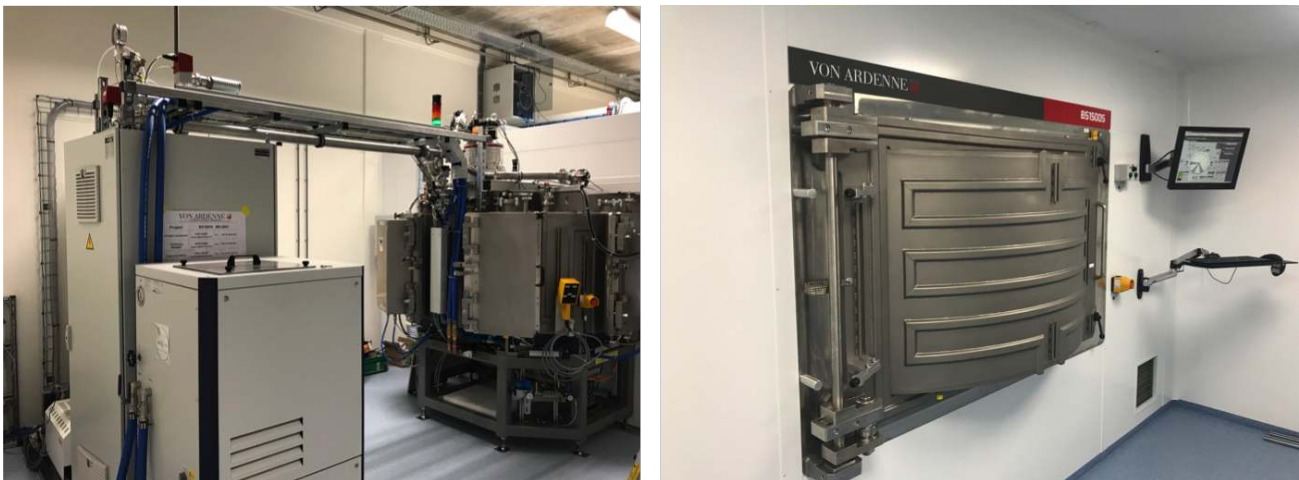
Figure 2: The fully operational ATHENA coating facility seen from the gray room (left) and the clean room (right).
