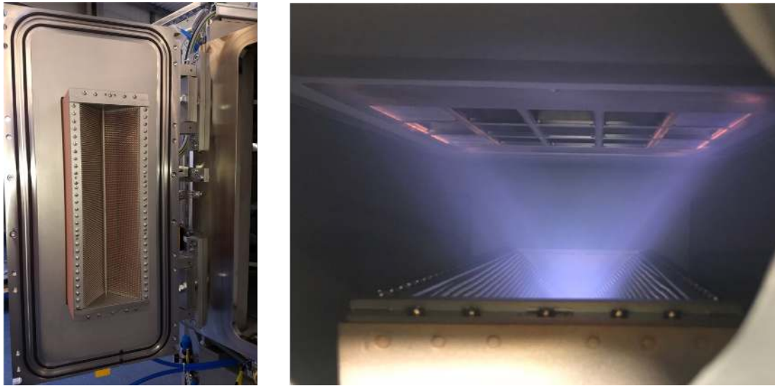
Figure 4: Left: Side view of the ISE. Right: Top view of a mirror plate plasma cleaning process performed in the BS1500S.
