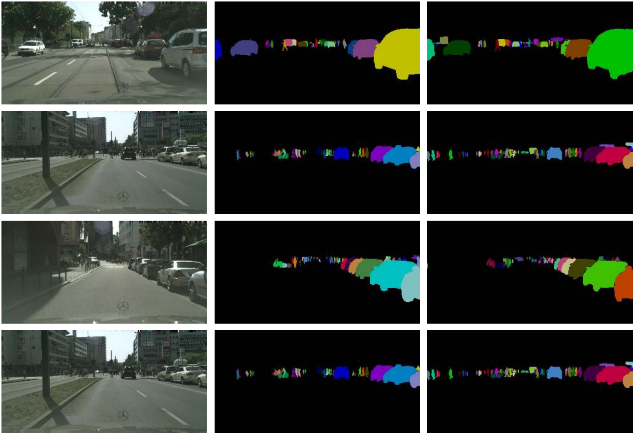
Figure 5. Results on the Cityscapes dataset. From left to right: input image, ground-truth and our predicts. Notice that our method is very good at detection small objects and often predicts more correct objects than annotated in the ground-truth.
