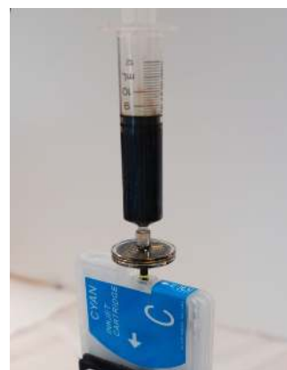
Figure 2. Filling an empty cartridge with conductive silver ink using a plastic syringe and disposable filter. Note that the ink is dark brown before it sinters.
