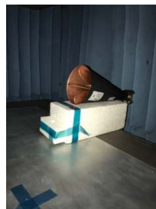
Figure 3.13. Round Feed Horn
