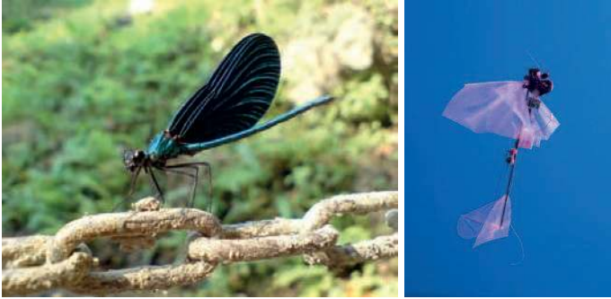
Figure 1.1: Damselfly (Beautiful Demoiselle, left ). Flapping micro air vehicle, DelFly II, in hovering flight ( right , de Clercq et al. 2009)
