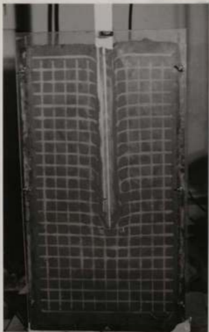
FIG. 15 DISTORTED GRID AFTER HIGH VELOCITY (2-662 FT/SEC) PENETRATION
