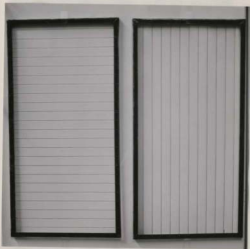
FIG-12 PHOTOGRAPH OF GRID FORMER OF CHORD TYPE
