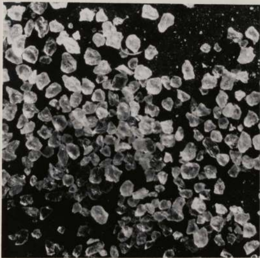
FIG 16A PHOTOGRAPHIC VIEW OF SILICA-70 SAND (MAGNIFICATION APPROX 40)
