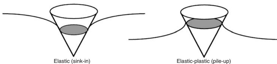
Fig. 5 Sink-in and pile-up during indentation
