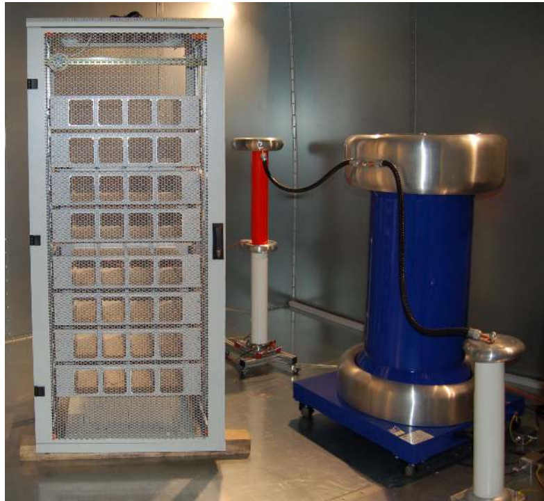
Fig. 8: PD test setup inside the Faraday cage.
