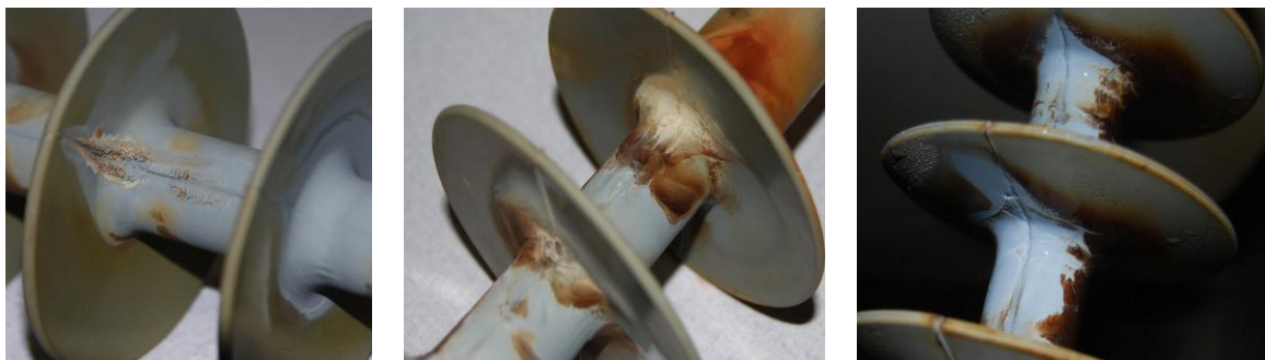
Figure 5.1: Comparison of material aging of the EPDM insulator for HVAC and positive and negative polarity HVDC excitation
