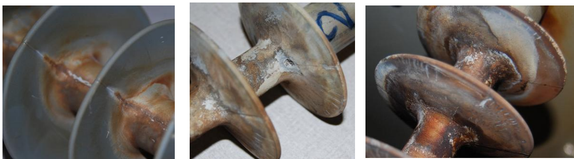
Figure 5.6: Comparison of aging for the HTV SR insulator (channel 2) for HVAC and positive and negative polarity HVDC excitation
