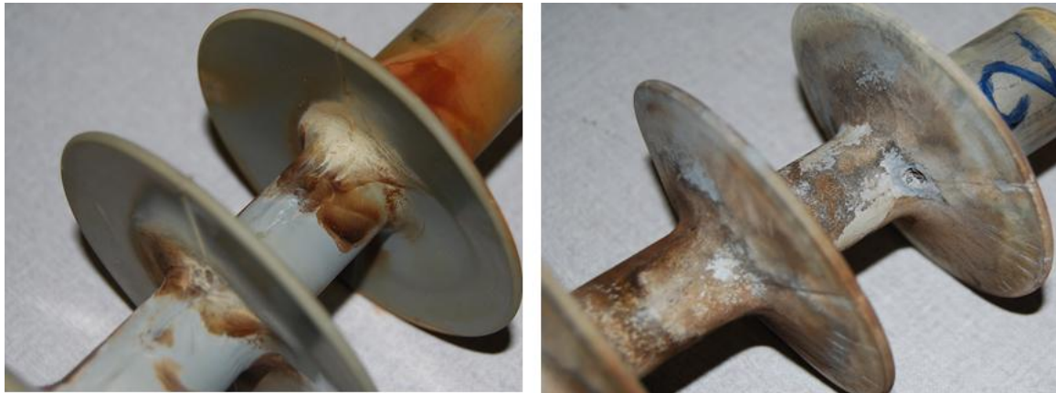
Figure 4.51: Comparison of aging of EPDM and HTV SR insulators for positive polarity HVDC excitation
