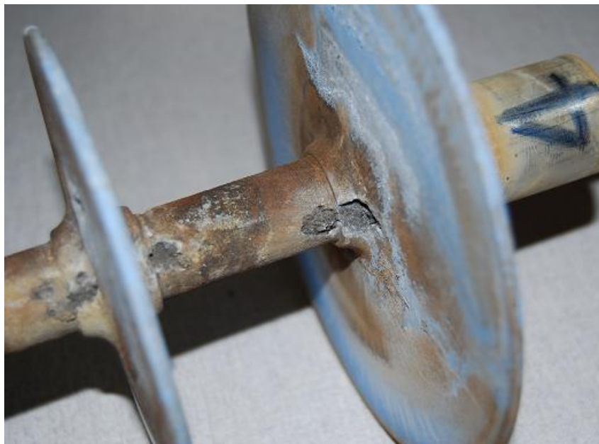
Figure 4.56: Detailed view of aging of the HTV SR insulator (Channel 4) for positive polarity HVDC excitation
