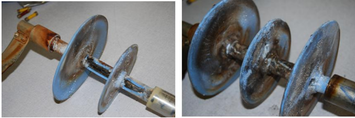
Figure 4.65: Wettability of the HTV SR insulator with a unified SCD of 28 mm/kV (Channel 3) and the HTV SR insulator with a unified SCD of 35 mm/kV (Channel 4)
