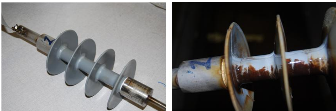
Figure 4.71: The EPDM insulator with a unified SCD of 28 mm/kV (Channel 1) before and after the test with negative polarity HVDC excitation
