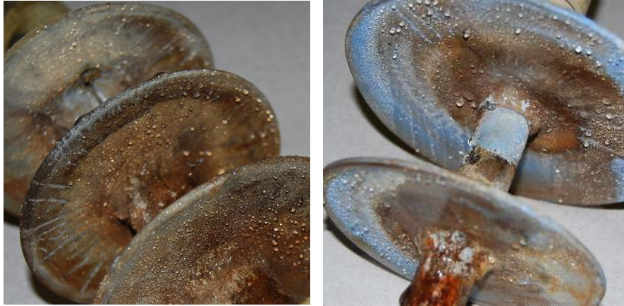
Figure 4.88: Wettability of the HTV SR insulators with a unified SCD of 28 mm/kV from manufacturer A (Channel 2) and from manufacturer B (Channel 3)
