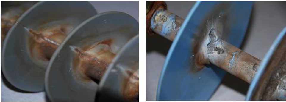
Figure 4.31: Comparison of aging of HTV SR insulators from manufacturer A and manufacturer B for HVAC excitation
