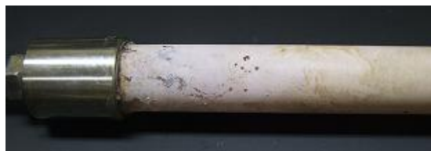
Figure 4.13: Visual aging of the RTV SR coated glass insulator with a creepage distance of 277 mm
