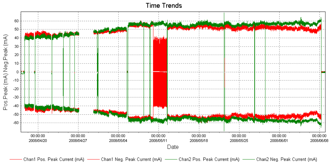
Figure 4.20: Peak leakage currents for the EPDM and HTV SR insulators for HVAC excitation
