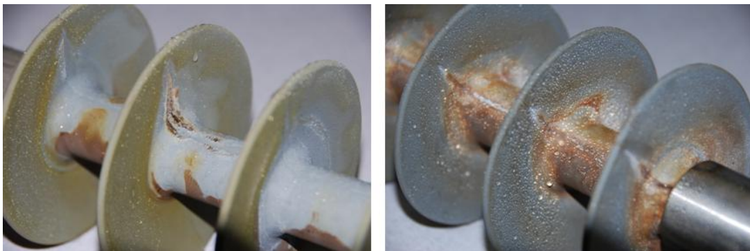
Figure 4.40: Wettability of the EPDM insulator (Channel 1) and the HTV SR insulator (Channel 2), both with a unified SCD of 28 mm/kV
