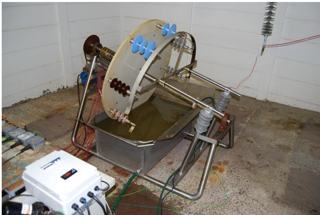
Figure D. 3: The Tracking Wheel Tester (TWT) with the fuse setup
