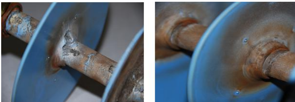
Figure 4.34: Comparison of aging of HTV SR insulators with creepage distances of 380 mm and 476 mm for HVAC excitation
