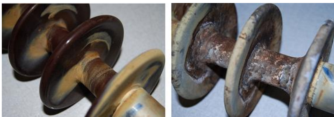
Figure 4.62: Comparison of aging of the porcelain and RTV SR coated porcelain for positive polarity HVDC excitation
