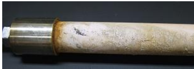
Figure 4.15: Visual aging of the RTV SR coated glass insulator with creepage distance of 433 mm
