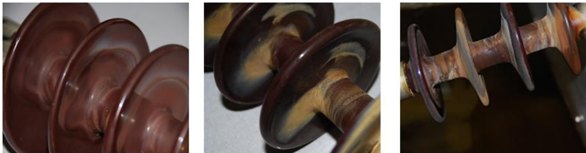
Figure 5.21: Comparison of material aging of the Porcelain insulator (channel 5) for HVAC and positive and negative polarity HVDC excitation
