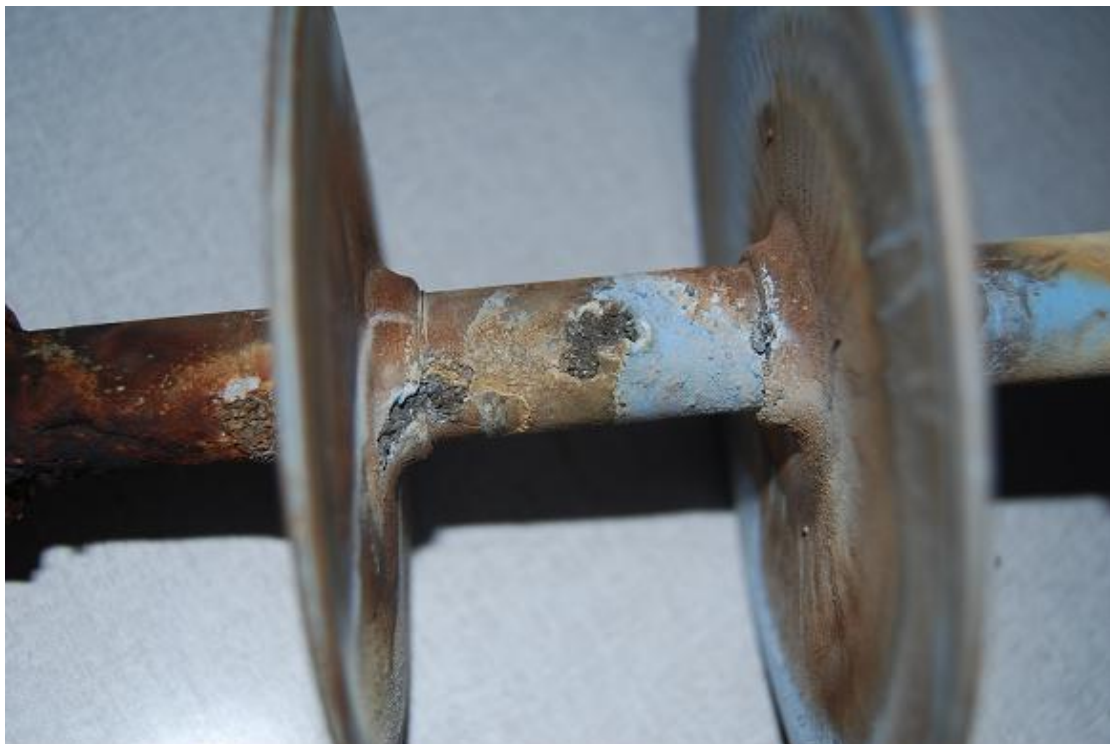
Figure 4.77: Detailed view of aging of the HTV SR insulator from manufacturer B (Channel 3) for negative polarity HVDC excitation
