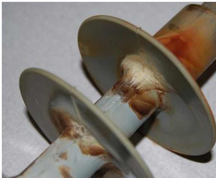
Figure 4.48: Detailed view of aging of the EPDM insulator (Channel 1) for positive polarity HVDC excitation
