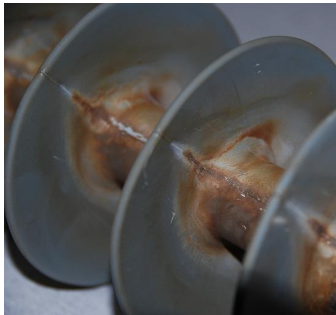
Figure 4.27: Detailed view of aging of the HTV SR insulator (Channel 2) for HVAC excitation
