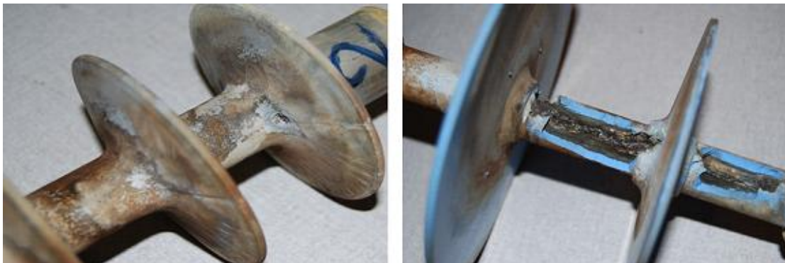
Figure 4.54: Comparison of aging of the HTV SR insulators from manufacturer A and manufacturer B for positive polarity HVDC excitation
