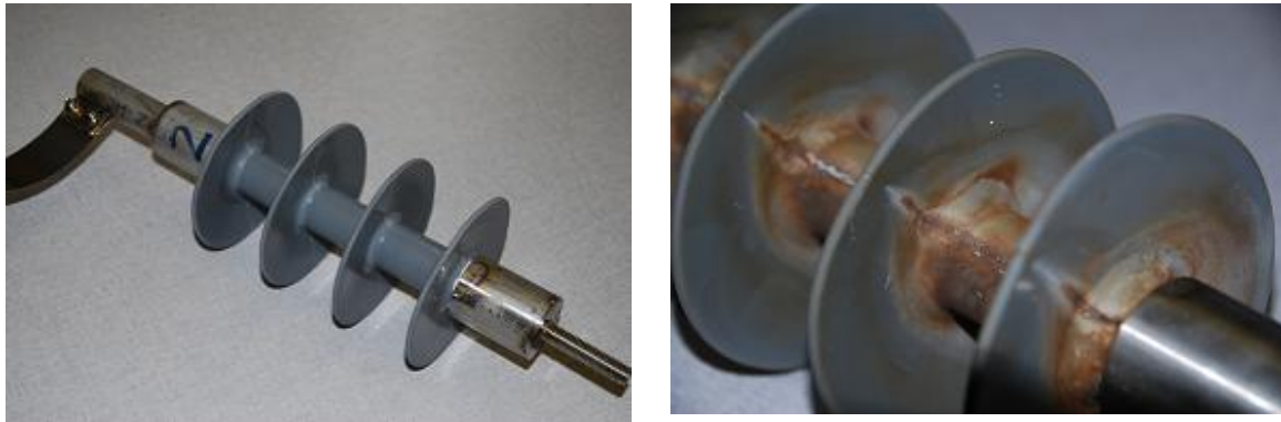
Figure 4.26: The HTV SR insulator (Channel 2) before and after the test for HVAC excitation
