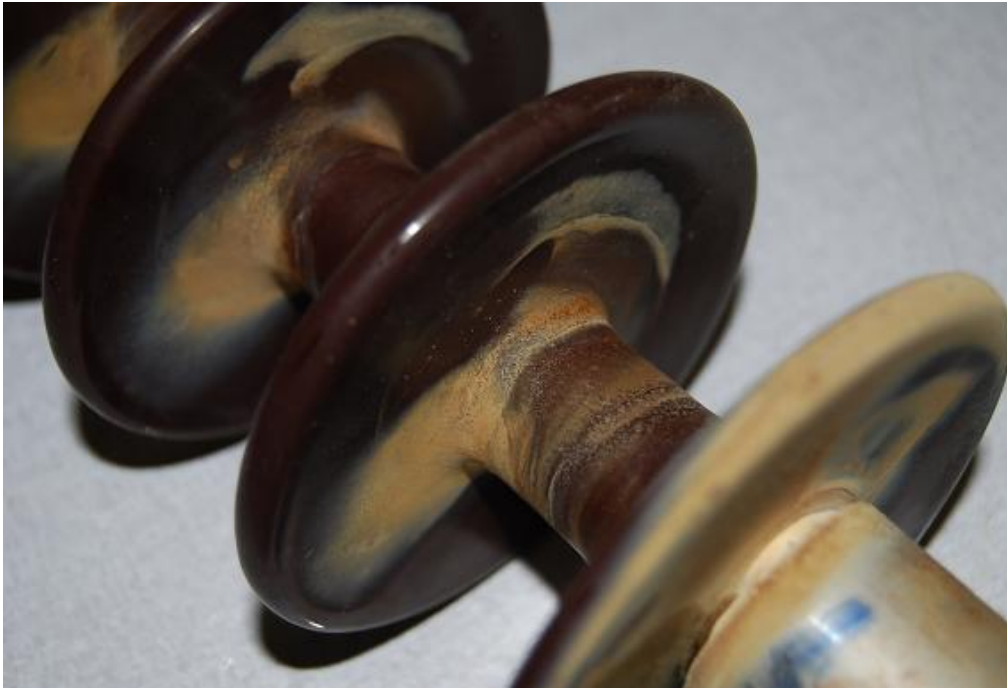
Figure 4.59: Detailed view of aging of the porcelain insulator (Channel 5) for positive polarity HVDC excitation
