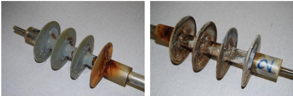
Figure 4.63: Wettability of the EPDM insulator (Channel 1) and the HTV SR insulator (Channel 2), both with a unified SCD of 28 mm/kV
