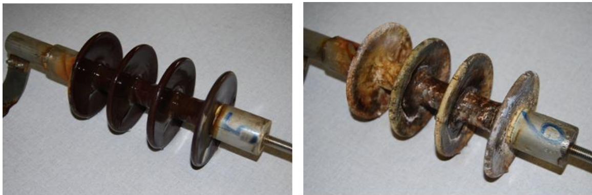
Figure 4.66: Wettability of the porcelain insulator (Channel 5) and the RTV SR coated porcelain insulator (Channel 6)
