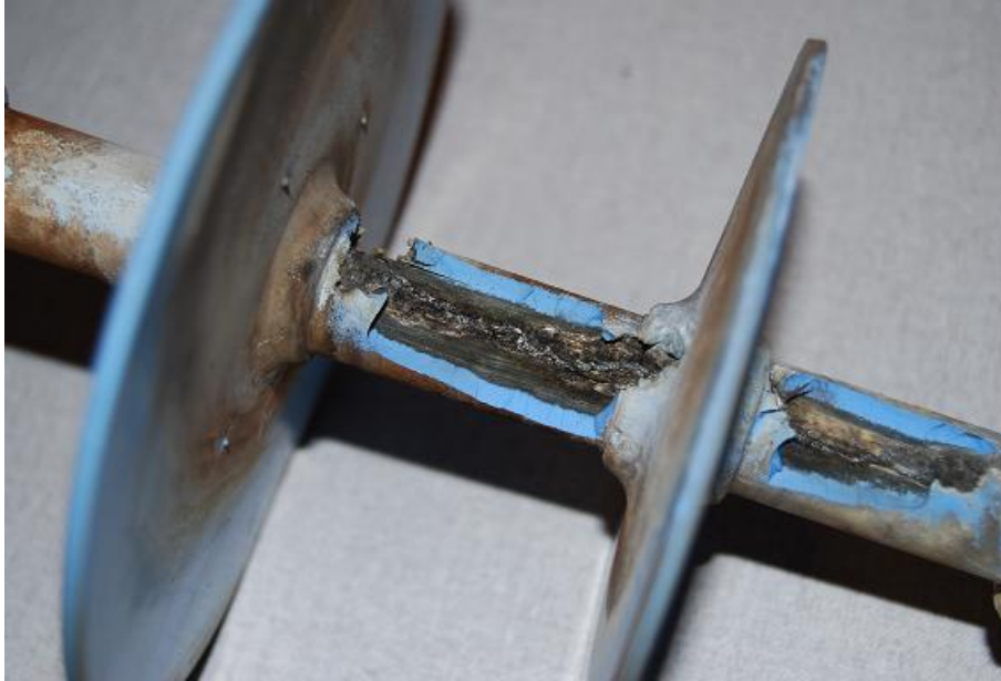
Figure 4.53: Detailed view of aging of the HTV SR insulator (Channel 3) for positive polarity HVDC excitation
