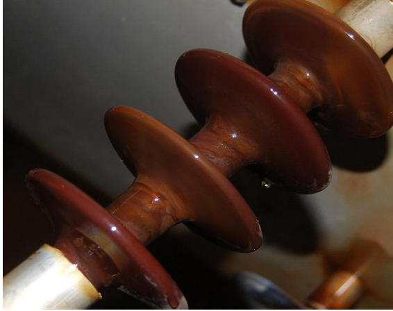
Figure 4.90: Wettability of porcelain insulator (Channel 5) and the RTV SR coated porcelain insulator (Channel 6)
