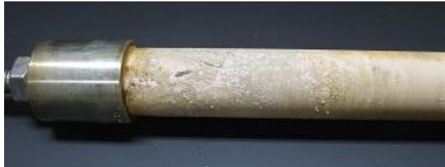
Figure 4.14: Visual aging of the RTV SR coated glass insulator with creepage distance of 346 mm
