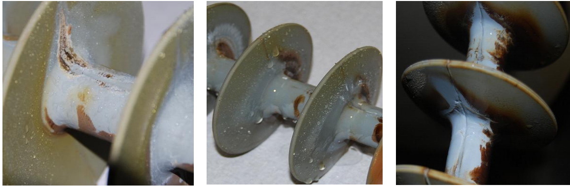
Figure 5.5: Comparison of hydrophobicity for the EPDM insulator (channel 1) for HVAC and positive and negative polarity HVDC excitation
