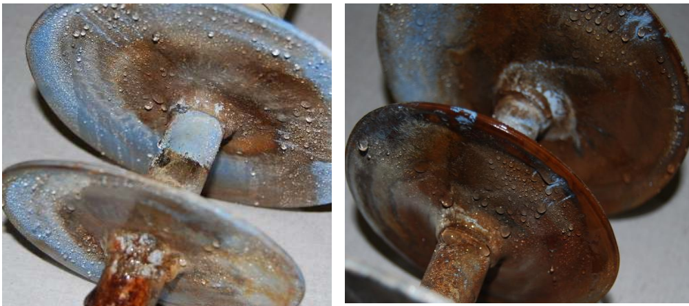
Figure 4.89: Wettability of the HTV SR insulators with a unified SCD of 28 mm/kV (Channel 3) and a unified SCD of 35 mm/kV (Channel 4)
