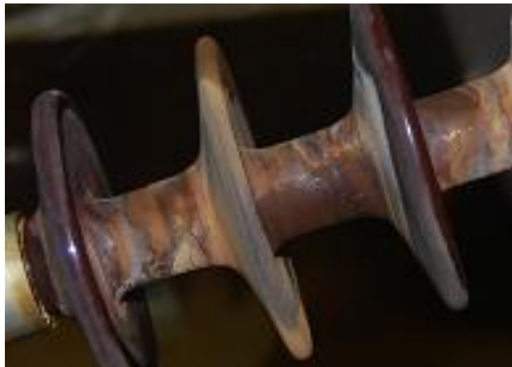
Figure 4.83: Detailed view of aging of the porcelain insulator for negative polarity HVDC excitation
