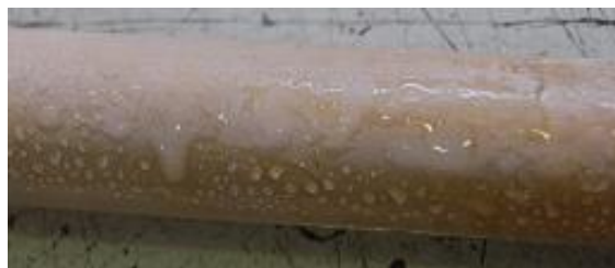
Figure 4.17: Wettability of the RTV SR coated glass sample with creepage distance of 346 mm (Channel 4)
