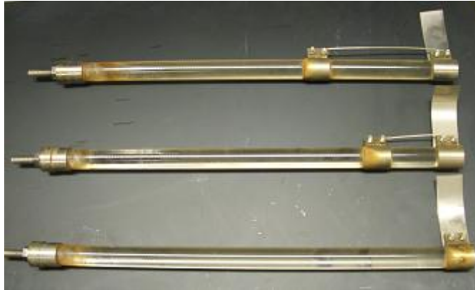
Figure 4.11: Visual aging of the glass samples
