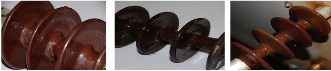
Figure 5.25: Comparison of hydrophobicity for the porcelain insulator (channel 5) with a unified SCD of 28 mm/kV for HVAC and positive and negative polarity HVDC excitation
