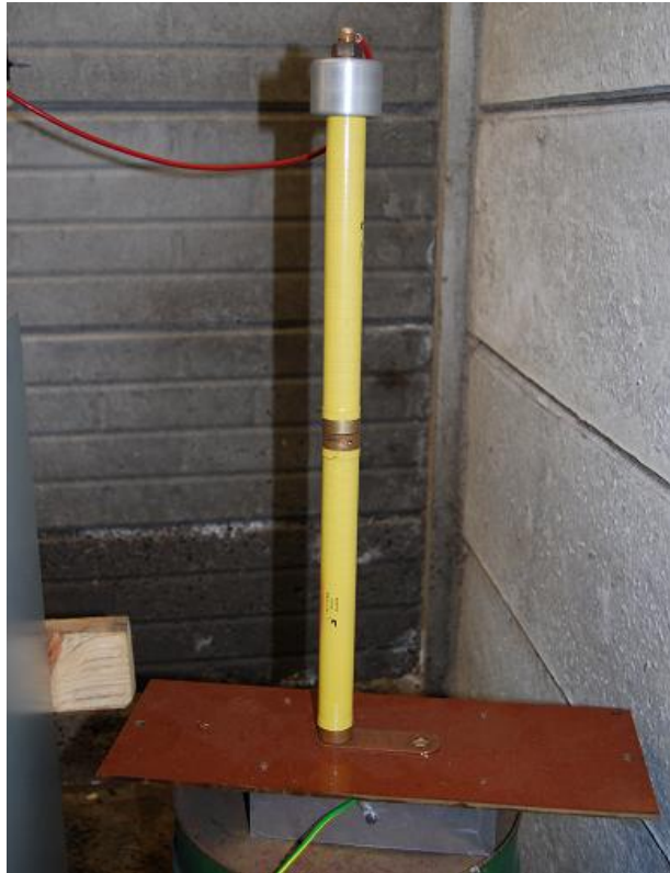
Figure D. 2: The voltage divider that was connected to the DC Source
