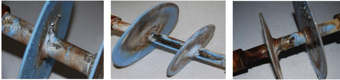
Figure 5.15: Comparison of hydrophobicity for the HTV SR insulator (channel 3) with a unified SCD of 28 mm/kV for HVAC and positive and negative polarity HVDC excitation
