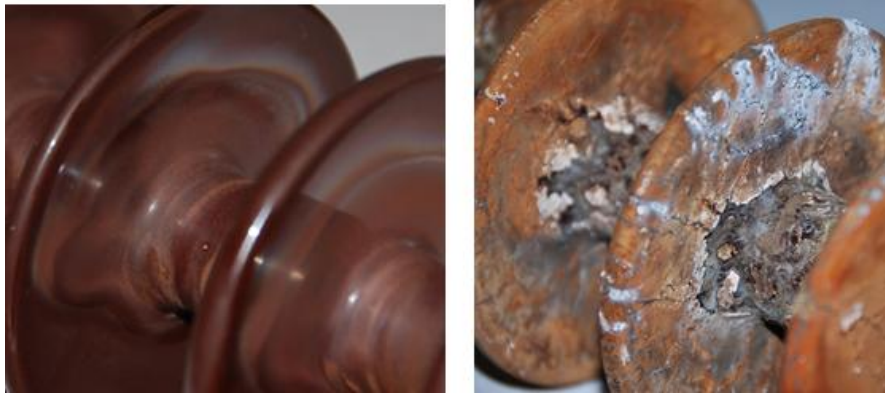
Figure 4.39: Comparison of aging of the porcelain and RTV SR coated porcelain insulators for HVAC excitation
