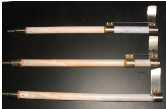
Figure 4.12: Visual aging of the RTV SR coated glass samples
