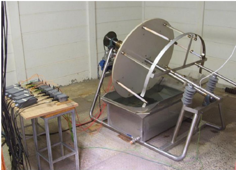
Figure 4.2: The tracking wheel tester with the test samples used in the first series of tests.
