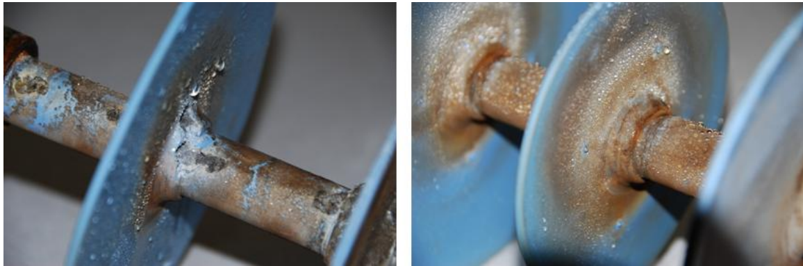
Figure 4.41: Wettability of the HTV SR insulator with a unified SCD of 28 mm/kV (Channel 3) and the HTV SR insulator with a unified SCD of 35 mm/kV (Channel 4)
