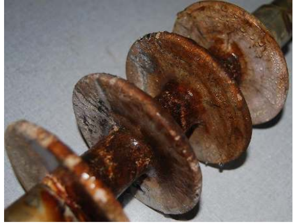
Figure 4.90: Wettability of porcelain insulator (Channel 5) and the RTV SR coated porcelain insulator (Channel 6)
