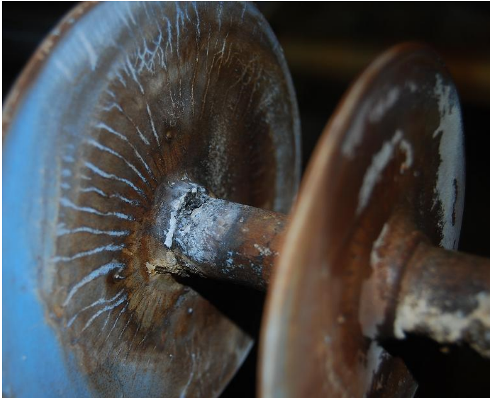
Figure 4.80: Detailed view of aging of the HTV SR insulator with a SCD of 35 mm/kV for negative polarity HVDC excitation
