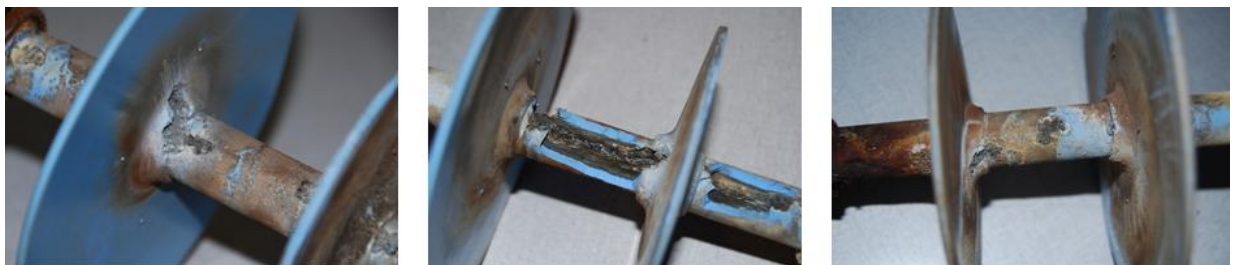
Figure 5.11: Comparison of aging for the HTV SR insulator (channel 3) with a unified SCD of 28 mm/kV for HVAC and positive and negative polarity HVDC excitation
