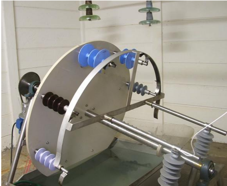
Figure 4.19: The Tracking Wheel Tester with the test samples used in the second series of tests with HVAC excitation.
