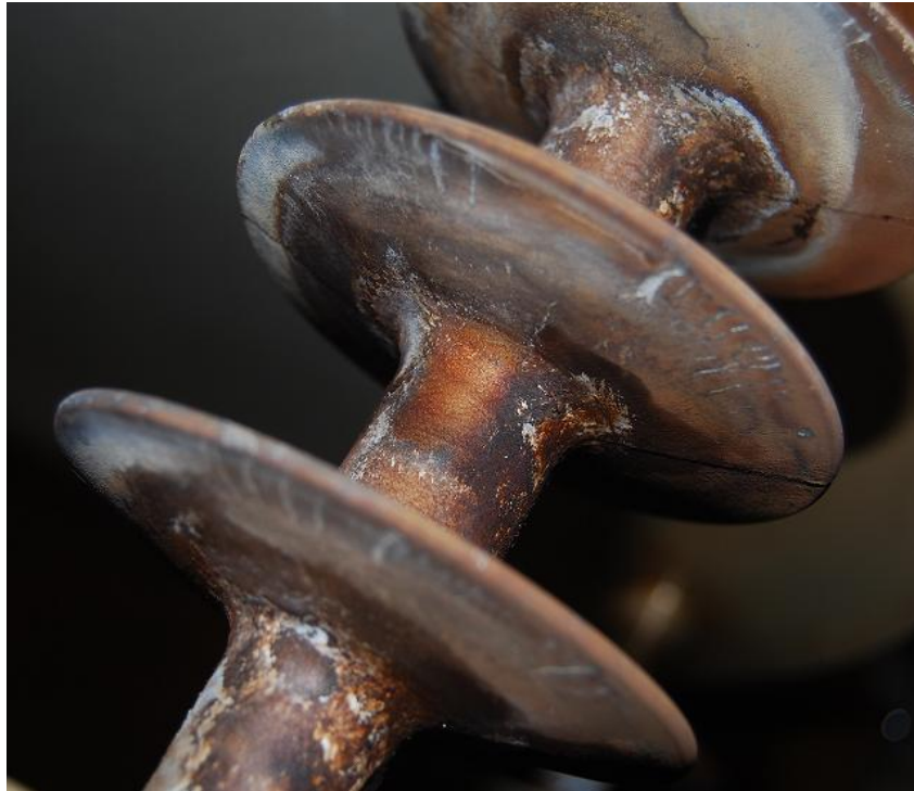
Figure 4.74: Detailed view of aging of the HTV SR insulator (Channel 2) for negative polarity HVDC excitation
