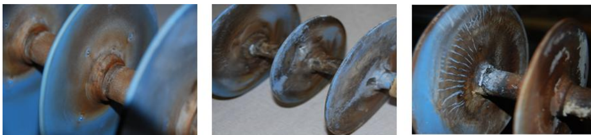
Figure 5.16: Comparison of material aging of the HTV SR insulator (channel 4) for HVAC and positive and negative polarity HVDC excitation
