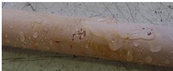
Figure 4.16: Wettability of the RTV SR coated glass sample with creepage distance of 277 mm (Channel 2)
