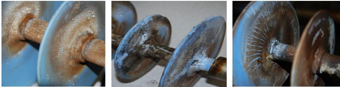
Figure 5.20: Comparison of hydrophobicity for the HTV SR insulator (channel 4) with a unified SCD of 35 mm/kV for HVAC and positive and negative polarity HVDC excitation
