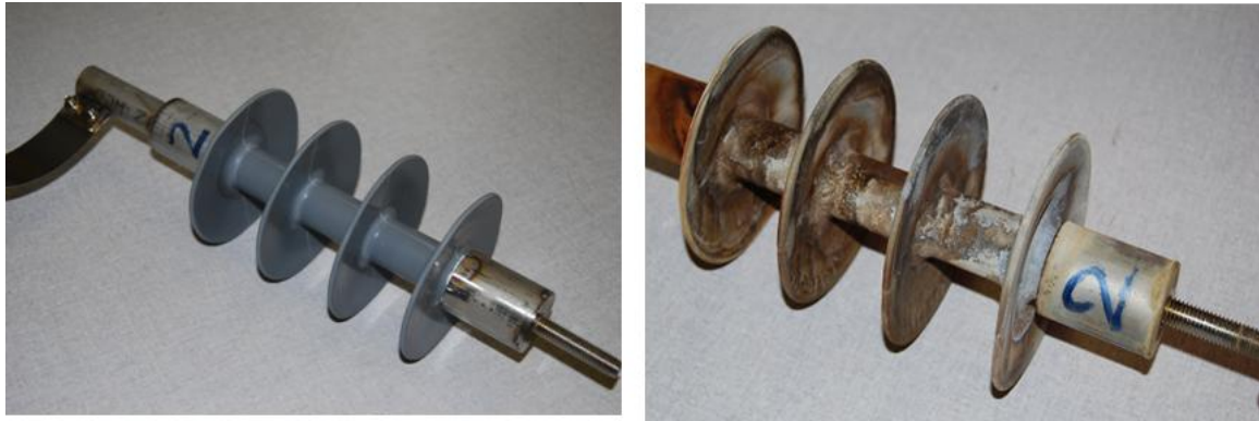
Figure 4.49: The HTV SR insulator with a unified SCD of 28 mm/kV from manufacturer A (Channel 2) before and after the test with positive polarity HVDC excitation
