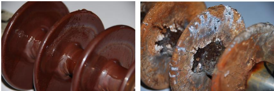
Figure 4.42: Wettability of the reference porcelain insulator (Channel 5) and the RTV SR coated porcelain insulator (Channel 6)
