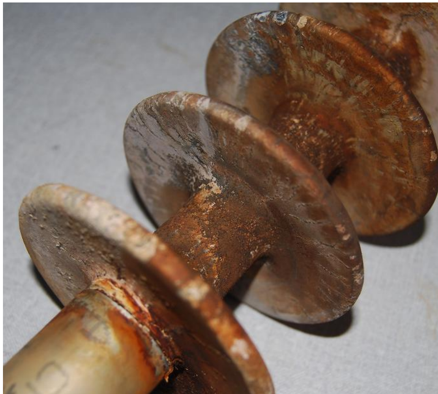
Figure 4.85: Detailed view of aging of the RTV coated porcelain insulator for negative polarity HVDC excitation
