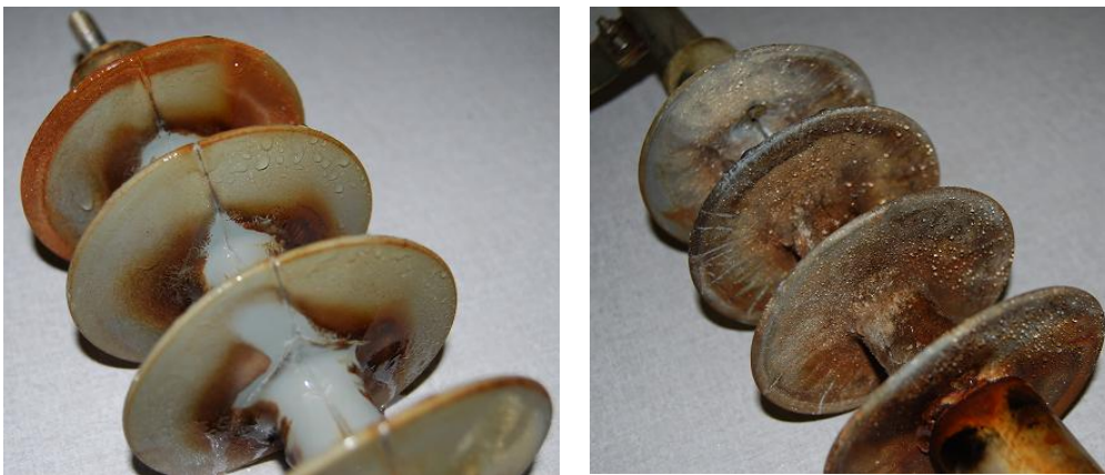
Figure 4.87: Wettability of the EPDM insulator (Channel 1) and the HTV SR insulator (Channel 2), both with a unified S_{CD} of 28 mm/kV
