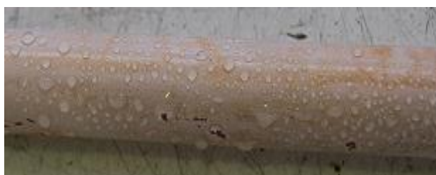
Figure 4.18: Wettability of the RTV SR coated glass sample with creepage distance of 433 mm (Channel 6)
