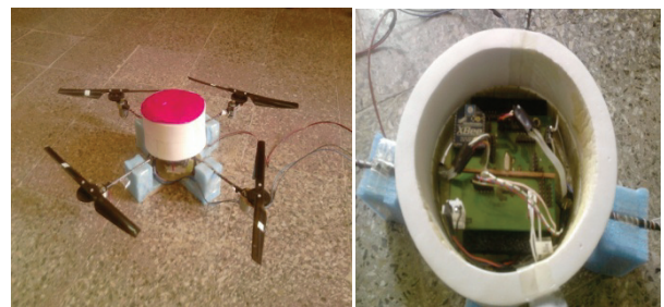
Fig. 8. The quadrotor with the embedded electronic and sensors
