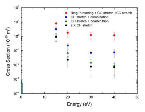
FIG 1. Integral cross sections  $(\times 10^{-20} \text{ m}^2)$  as a function of incident electron energy for excitation of the (a) ring puckering + CO stretch + CC stretch (red diamond), (b) CH stretch + combination (blue square), (c) OH stretch + combination (green triangle), and (d) CH stretch overtone (black circle) composite vibrational-modes in phenol. See also legend in figure.
