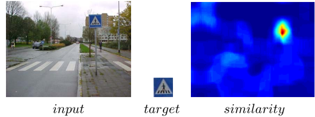
Figure 5. Object detection using a 2^{15} -bins color histogram. The computed similarity map is same as the conventional approach; however the integral histogram method runs in 63msecs although the conventional exhaustive search takes approximately 2 minutes for 100 scales on a 3.2Ghz P4.
