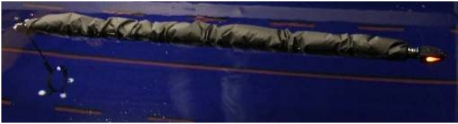
Fig. 13. The underwater snake robot Mamba in the pool with the markers attached on the tail for position measurements.
