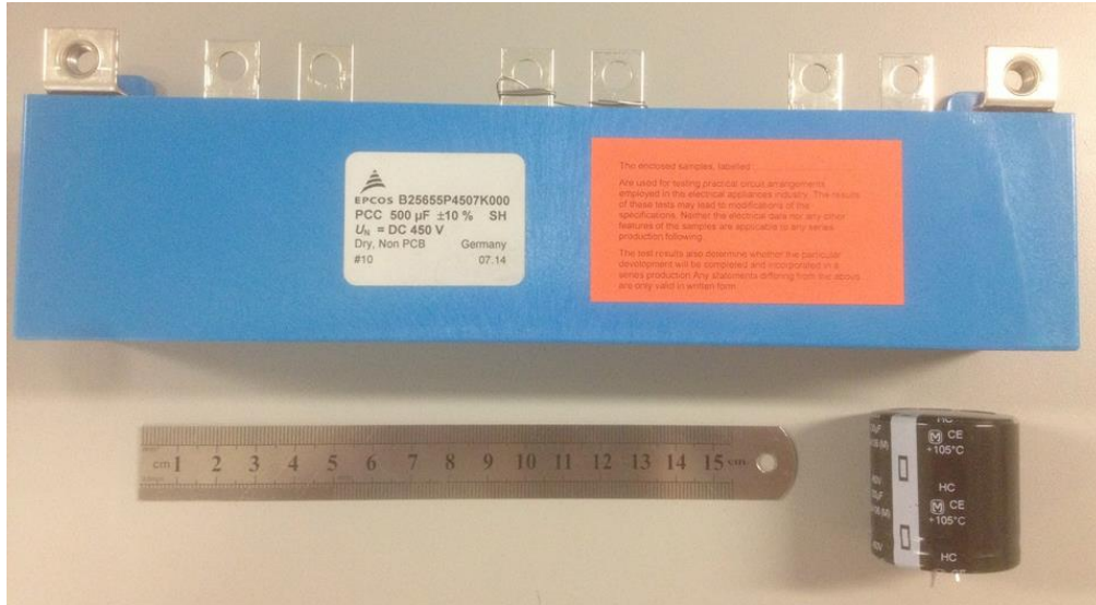
Fig. 1.10. A comparison between 500 \mu\text{F}/450\text{ V} film capacitor and a 330 \mu\text{F}/450\text{ V} electrolytic capacitor.
