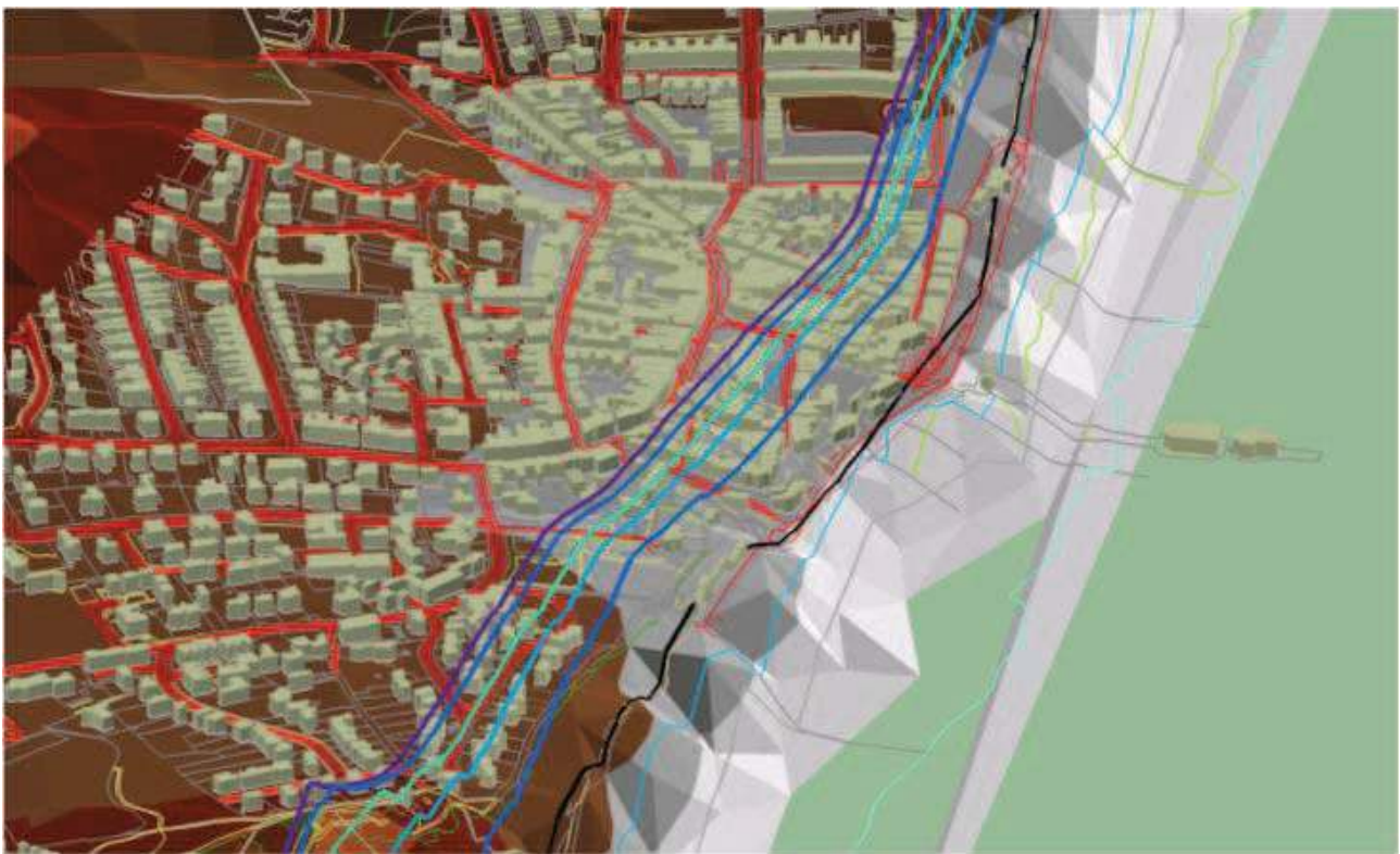
Figure 19 Virtual reality visualisation of coasts (each line represents a 10 year central estimate of the cliff toe position)
