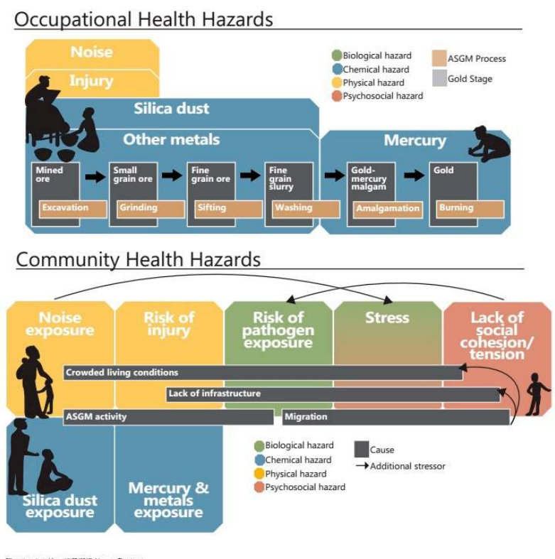
Figure 2. Key occupational (top panel) and community (bottom panel) human health hazards in the Ghanaian artisanal and small-scale gold mining (ASGM) sector. Silhouettes adapted from UNEP Mercury: Time to Act (2013) [22].
