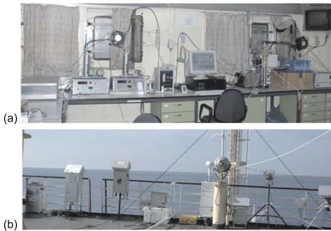
Figure 2. (a) Photograph of the aerosol and gas laboratory on the B deck of the ORV showing the different instruments connected to the community air inlets. (b) An array of outdoor aerosol instruments on the B deck sampling into the incoming air.
