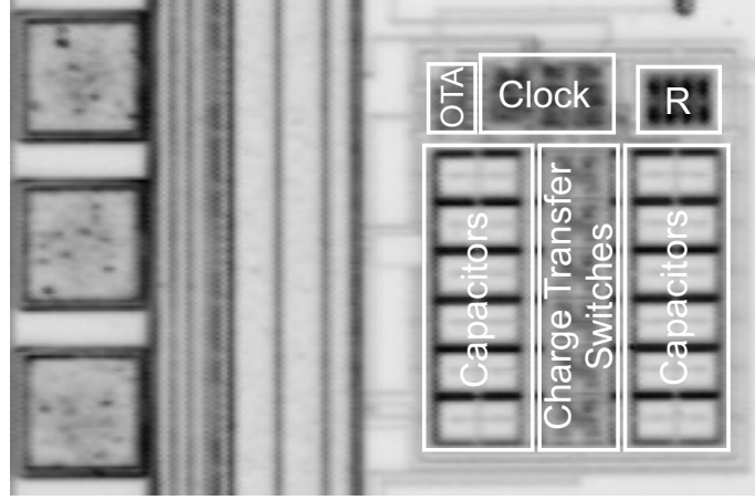
Figure 3.9: Die photograph of the complete regulated charge pump circuit. The size is 230\mu\text{m} \times 300\mu\text{m} .
