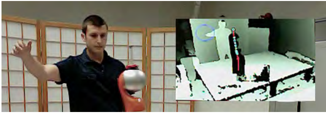
Fig. 5. Snapshot of a collaboration experiment. In the box on the right, the associated depth image shows, highlighted by a blue circle, the collaborative human part (the right hand) that has been removed
