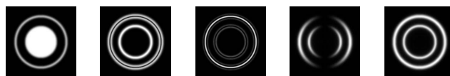
Figure 2: Left to right: original image (circular step and roof edges); gradient magnitude; squared Laplacian; oriented quadrature filter; boundary energy. Only the boundary energy yields a rotational invariant unimodal response for both step and roof edges. Filtering is done in the Fourier domain throughout the paper.
