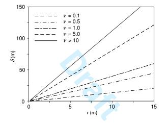
FIG. 1. Relationship between scale of fluctuation,  $\delta$ , and Matérn function parameters,  $\nu$  and r
