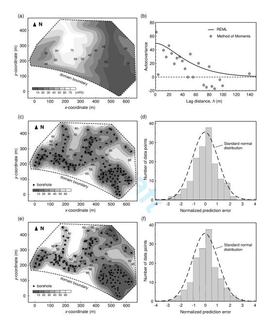
FIG. 3. (a) Rockhead level; (b) Autocovariance structure; (c,d) Prediction variance contour and normalized prediction errors in transformed space; (e,f) Prediction variance contour and normalized prediction errors in back-transformed original space
