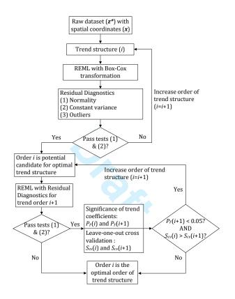
FIG. 2. Flowchart of integrated residual analysis framework
