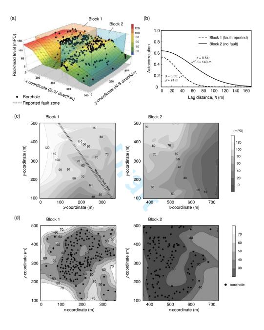
FIG. 6. (a) Two sub-regional blocks at CWE site; (b) Autocorrelation structures for two blocks; (c) Variations in rockhead levels; (d) Prediction variance contours for two blocks
