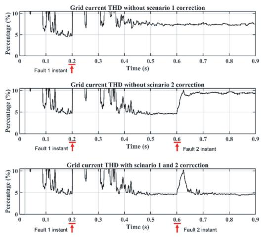
Fig. 18. Impact of the M-IFS-MPC on grid current THD: (a) without Scenario 1 correction. (b) without Scenario 2 correction. (c) under M-IFS-MPC correction.
