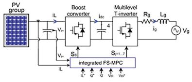
Fig. 8. Proposed integrated FS-MPC for PV-GCS.
