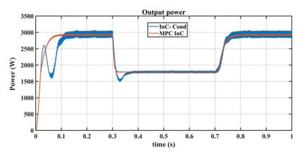
Fig. 5. Performance of MPC Inc-Cond against Inc-Cond under sudden change of illumination.
