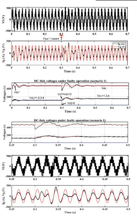
Fig. 14. Results for Scenario 1 (DC-link capacitor short-circuited): Output voltage, voltage and grid current, DC-link voltages with their zoom.
