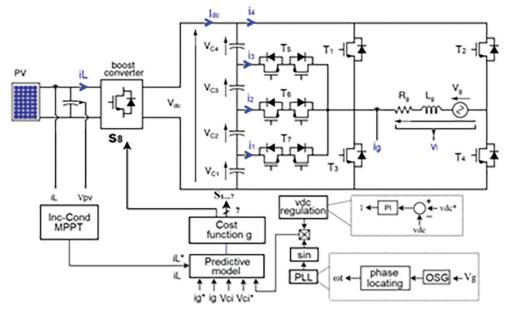
Fig. 10. Control scheme of the proposed PVGCS using FS-MPC.
