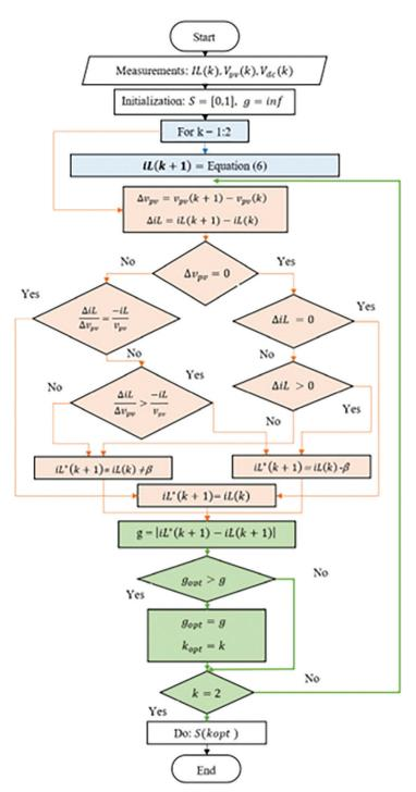
Fig. 6. Flowchart of the hybrid predictive Inc-Cond control.
