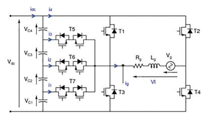
Fig. 4. Power circuit of the five-level T-type inverter.
