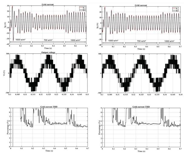
Fig. 11. Simulation results for separated and integrated FS-MPC (DC-link capacitor regulation, grid current and output voltage with grid current THD). FS-MPC, finite set-model predictive control.
