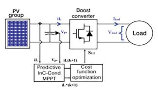
Fig. 3. Hybrid predictive Inc-Cond MPPT control scheme.
