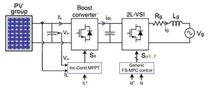
Fig. 1. General PVGCS scheme using FS-MPC control.
