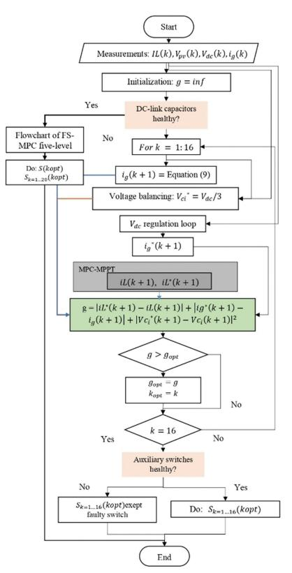
Fig. 15. Flowchart of the proposed M-IFS-MPC for the faulty mode of the power converter.
