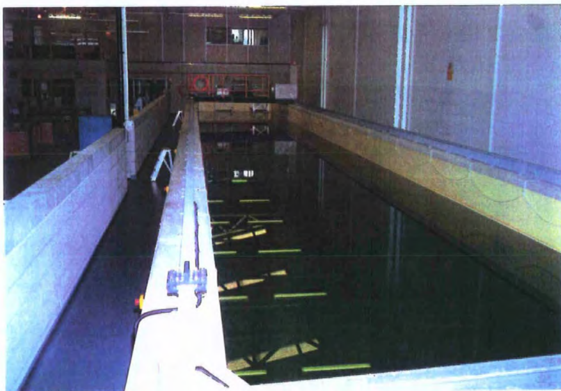
Plate 5.2. Towing tank at the Royal Naval Engineering College.
