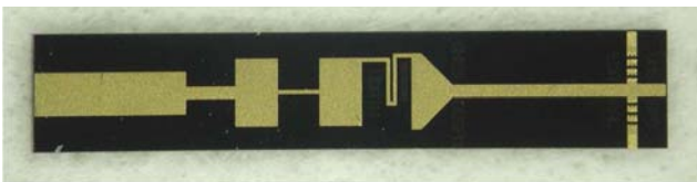
Fig. 1 Optical image of a 190 GHz doubler circuit (total length 1.8 mm).
