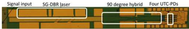
Fig. 6. A microscope picture of PIC integrating SG-DBR laser, star coupler, photodetectors, and microstrip transmission lines [63].
