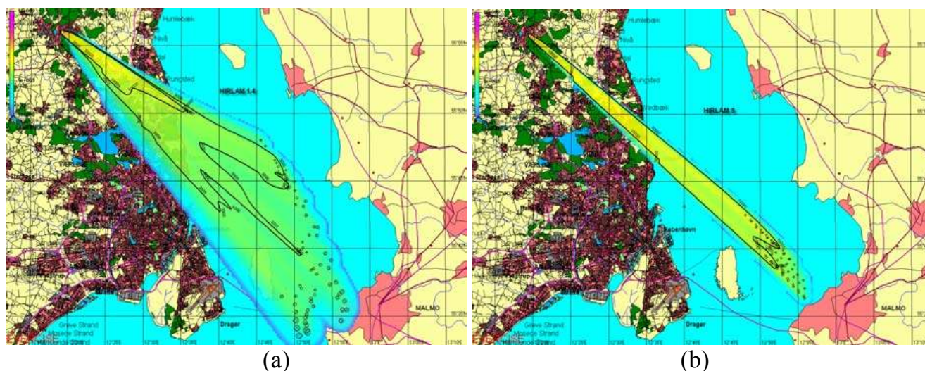
Fig. 8. A local-scale plume from the ^{137}\text{Cs} hypothetical atmospheric release in Hillerød at 00:00 UTC, 19 June 2005 as calculated with RIMPUFF using DMI-HIRLAM and visualised in ARGOS for the Copenhagen Metropolitan Area. Cs-137 air concentration for different DMI-HIRLAM data: (a) urbanised U01, 1.4 km resolution, (b) operational S05, 5 km resolution.
