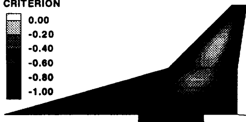
D) PANEL BUCKLING LENGTH 2FT
