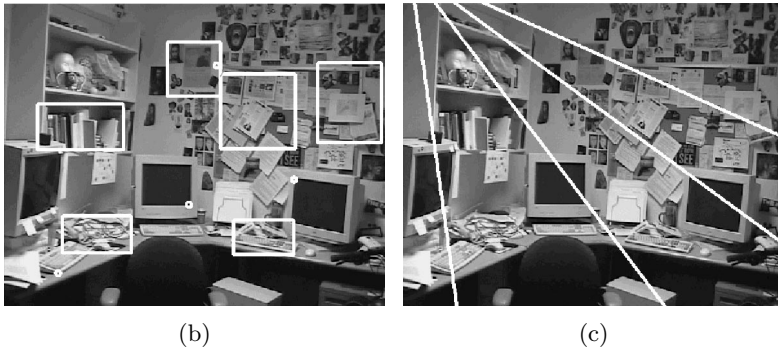
Fig. 4. First (a) and last (b) images in a 6-frame sequence. The rectangles represent the manually selected patches. A “direct multi-frame” algorithm was used to estimate the affine motion parameters of every patch throughout the sequence. The affine parameters are used to recover the epipoles directly . The fundamental matrix is recovered from the epipoles and an arbitrary legitimate homography only to visualize the epipolar lines. We show the quality of the fundamental matrix on a number of hand-selected points. Note that the epipolar lines pass near the matching points.
