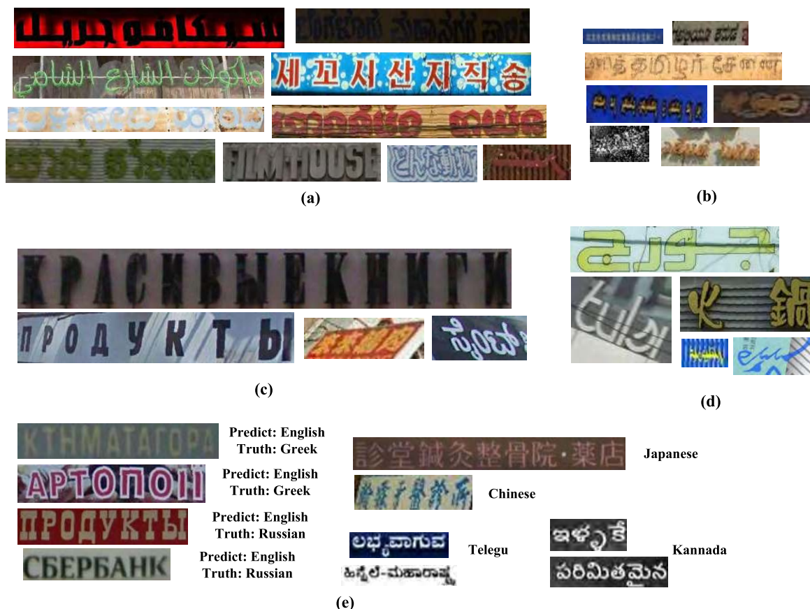
FIGURE 8. Samples that our approach fails to identify. (a) Complex background or background and text mixed together. (b) poor quality text. (c) Large text spacing or non-horizontal text. (d) shelters in front of text. (e) Great similar scripts such as Russian, Greek and English; Japanese and Chinese, Telegu and Kannada.
