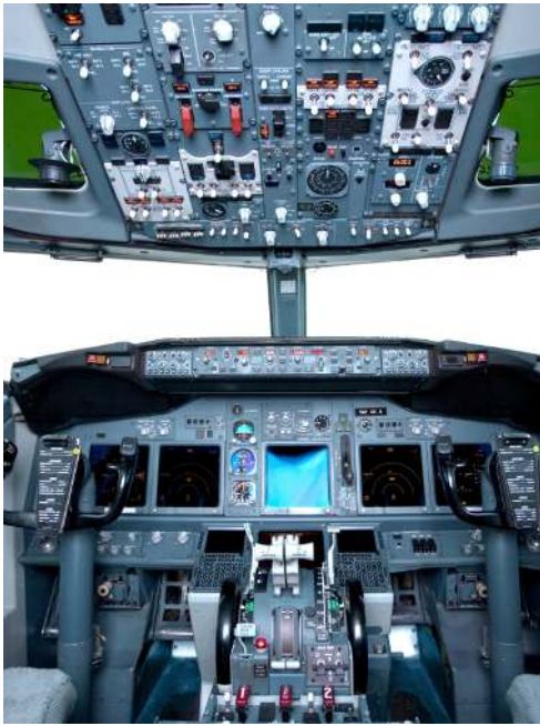
Figure 3. Our testbed: view of a Boeing 737 cockpit. This image was printed in size 3'×4' and mounted to a metal panel on the wall. The resolution is high enough that most of the control element labels are readable. Original image file obtained from iStockphoto.com/Smaglov.
