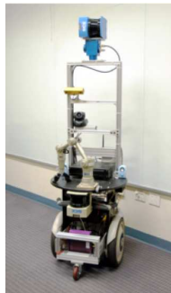
Fig. 1. Our robotic platform, hardware specifications, and data flow: a sparse point cloud is reconstructed in software by knowing the relative pose between the pan/tilt unit and the video camera, and correcting for robot motion using odometry. The depth of every pixel is then inferred, and features from the 2-d image and the 3-d point cloud are combined by our probabilistic object detectors.
