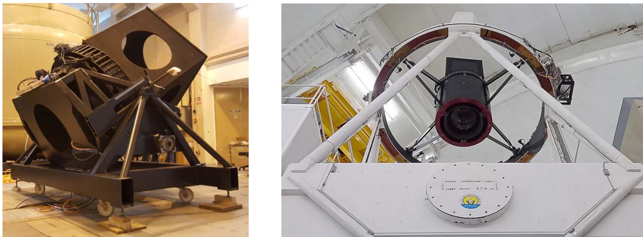
Figure 2 (left) The PFR under test in the WHT dome. (right) The corrector installed in the top end and ready for testing on-sky.
