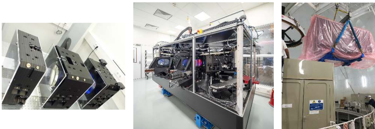
Figure 7: (left) Lens groups of the red camera during integration. (center) The complete spectrograph under test in the lab at ASTRON. (right) The spectrograph being lifted into the GHRIL enclosure.
