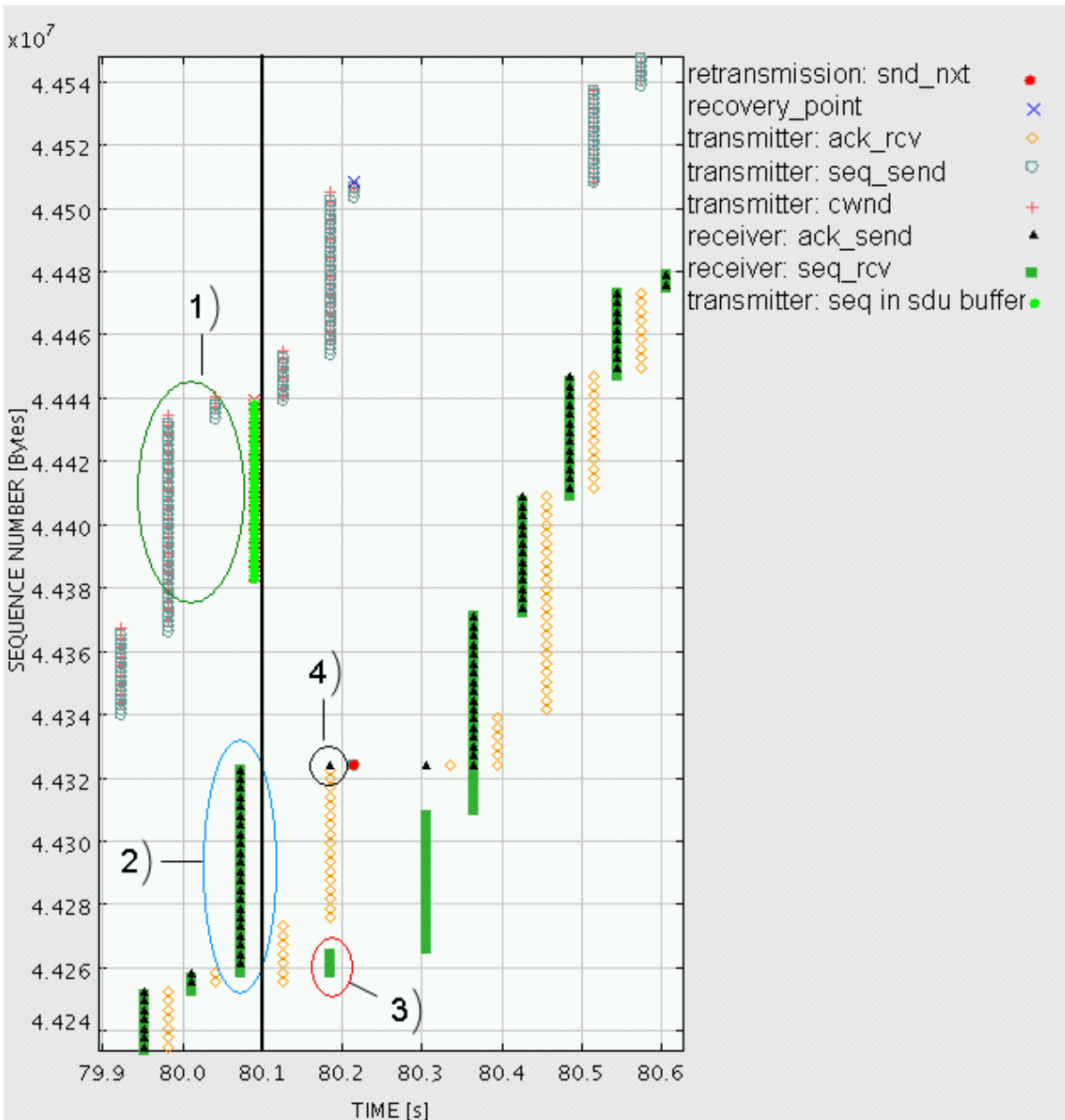
Figure 6.65 : TCP trace of fast recovery for SDU reconstruction (access handover marked with line).
